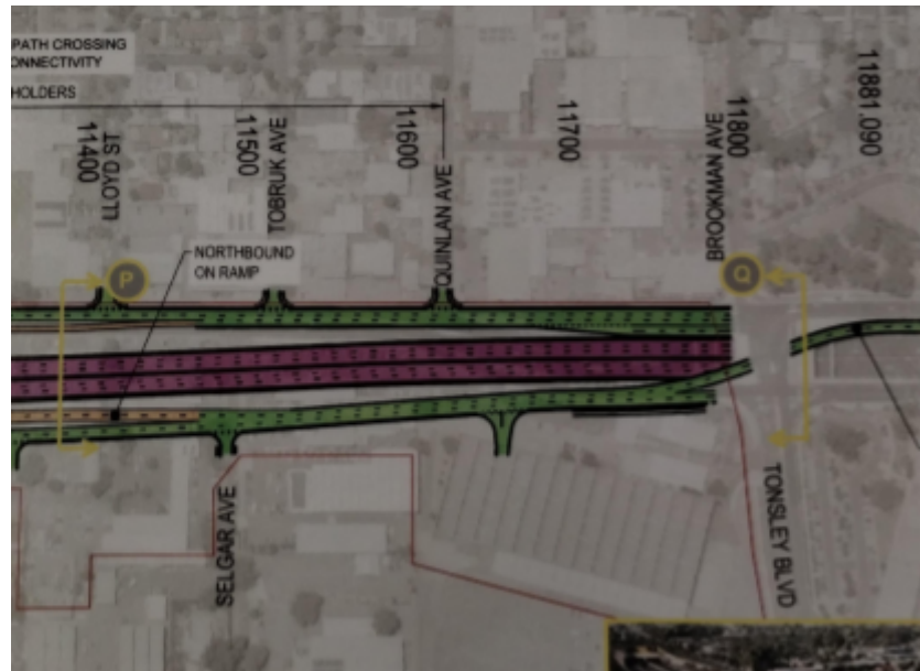
Section of the approach to the southern tunnel from the south, as shown on a drawing displayed at a community information session in February 2023 (this is a photo of that drawing). The tunnel entrance is off the left of this image, but observe how much wider the road gets as it approaches it, compared to the existing Darlington motorway shown on the right of this image.
